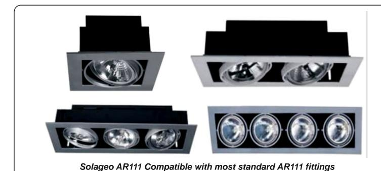
Luminous Color **Power Beam** Model **Dimensions** Lifespan Wattage Current **Base** Flux **Factor Angle Temperature** Ext. Diameter x **Model Code** degrees W pf Amp lm Type **Hours** Height, mm LAR10WSS-COB-3 10 >0.5 0.07A 810 120° 3000K G53 112x58mm 30,000 LAR10WSS-COB-6 10 >0.5 0.07A 810 120° 6400K **G53** 112x58mm 30,000
